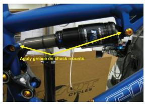
Install long shock bolt using anti-seize and torque to (10lb. ft, 120lb. in, 13Nm.) Install short shock bolt. Use blue loctite on the M5 bolt. Torque M5 bolt to (5lb.ft, 60lb.in, 7Nm.)
