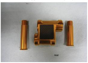
Use anti-seize and torque link pins to (27lb ft, 35 Nm.)
