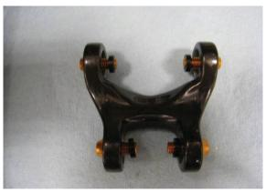
Install rocker bolts using grease or anti-seize. Torque to (10 lb.ft, 120 lb.in, 13 Nm.)
